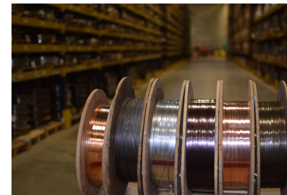
Shown from left to right: Beryllium Copper, Carbon Steel, Stainless Steel, Carbon Steel, Phosphorus Bronze, and Inconel
