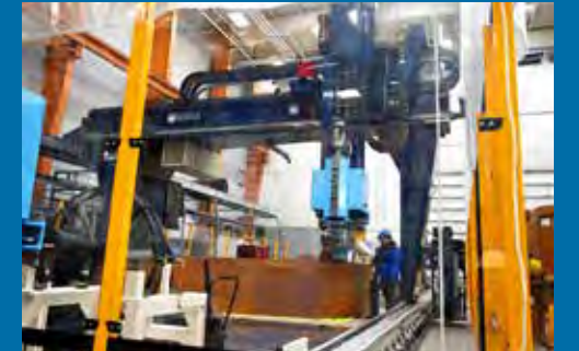
A new composite of wood and biopolymers can be extruded into components for cheap and durable new homes. Photo: University of Maine
