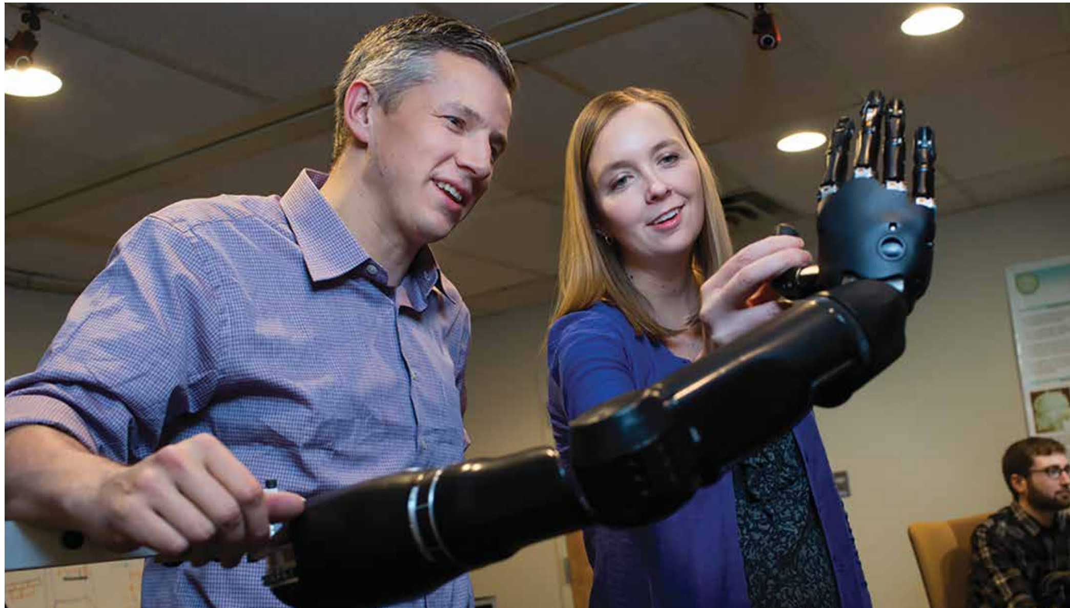
Robert Gaunt and Jennifer Collinger are researching brain-computer interface technology for individuals with motor impairments, including devising this neuroprosthetic limb.
